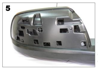
5. This is the back of the mirror housing after you have completed removing the old cap.
